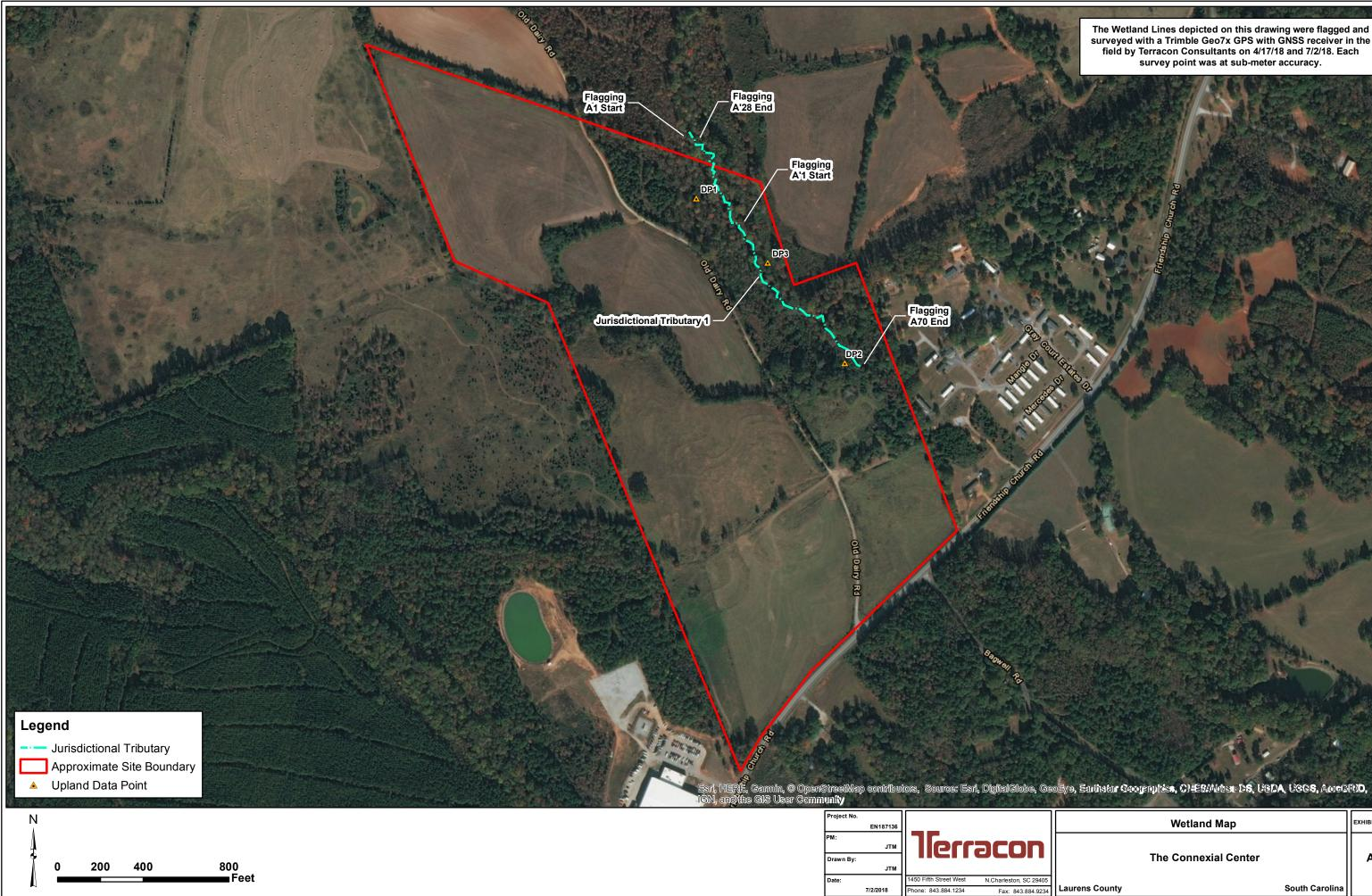
The Wetland Lines depicted on this drawing were flagged and surveyed with a Trimble Geo7x GPS with GNSS receiver in the field by Terracon Consultants on 4/17/18 and 7/2/18. Each survey point was at sub-meter accuracy.
